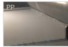
delamination due to a missing layer
