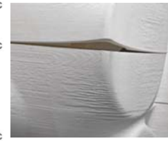
delamination due to a missing layer
